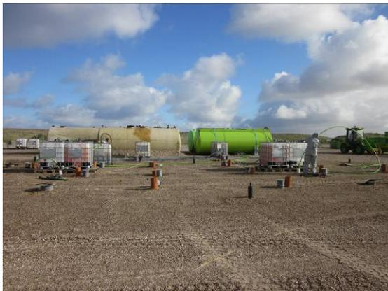
It was possible to extract approx. 50 m<sup>3</sup> of groundwater from each cell which is equivalent to 40% of the estimated total water content in a test cell. It is estimated that approx. 50% of the water in the test cell are drainable, e.i. approx. 80% of the "drainable water" was removed. The infiltration of the caustic soda solution by gravitation was successful, however pH measurement showed that caustic soda was not fully distributed to the upper layers of the test cells.
