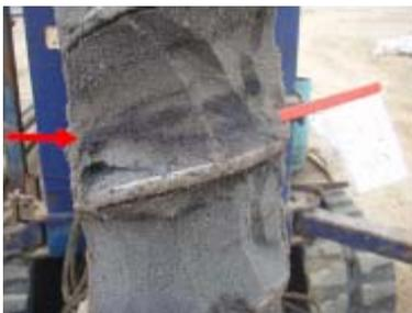
The presence of free mobile organic phase was observed on top of the silt layer in approximately every 3rd well in the test cells. In addition, residual free phase (dark NAPL not flowing freely from the soil sample) was observed in three wells.
