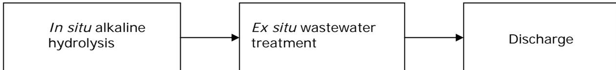
Figure 1: Conceptual model for treatment train of envisioned remediation at the site. The NorthPestClean project focuses on the *in situ* alkaline hydrolysis
