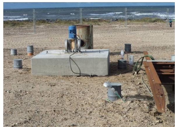
an *ex situ* and an *in situ* vibration source. The results from sweep tests have been reviewed to assess the equipment, frequency, and amplitude that best transmit the vibration energy from a seismic source to the target area. The preliminary tests showed that vibration induced from the topsoil (*ex situ*) was just as efficient as an *in situ* source. As a result of the pre-test a device was constructed to deliver a frequency around 43 Hz and amplitude at approx. 30 kN.
